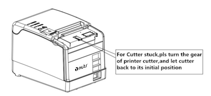
Note: do not open cover by force, or may cause unrecoverable damage to the print head and the cutter.
