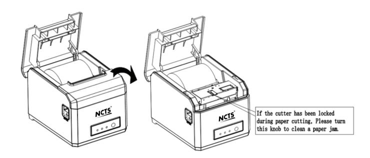
Note: do not force open the cover, as to avoid unrecoverable damage to the print head and the cutter
